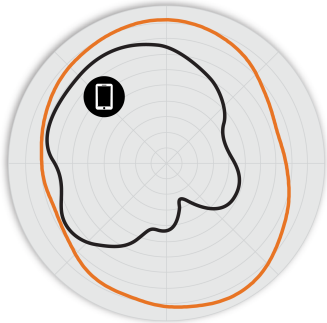
Figure 2. H350 2.4GHz Azimuth Antenna Patterns
