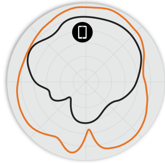
Figure 3. H350 5GHz Azimuth Antenna Patterns
